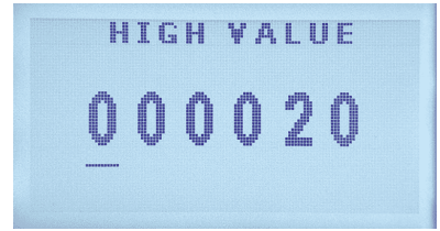
Fig. 29 - Span Setting - 20mA
