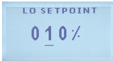
Fig. 19 - Relay 1 Low Set Point
