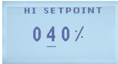
Fig. 18 - Relay 1 High Set Point
