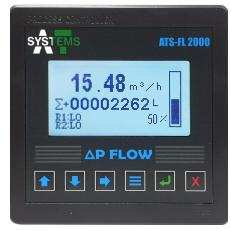
ATS-FL2000 is an industrial standard flow controller which is directly compatible to FT-1000 flow transmitters. ATS-FL2000 flow controller is simple to install in any industrial panel and fits in a 96mm x 96mm cutout. The flow controller comes with built-in 8 digits digital totalizer offering different unit selection. It has a built-in micro-SD card for storing flow and sum values with time.
