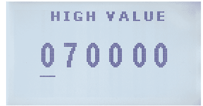
Fig. 26 - Span Setting - 20mA
