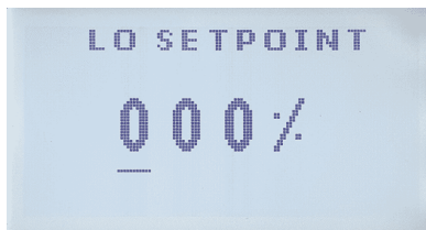
Fig. 19 - Relay 1 Low Set Point
