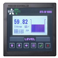
ATS-LV1000 Level Controller is an industry standard controller used for monitoring, analyzing, logging and controlling fluid level in a tank. With a wide range of user selectable tank shapes, dimensions, display units, relay settings and sensor and medium specifications, it provides an enhanced user experience. Built-in micro SD card for data acquisition and communication with the custom built desktop application add a dynamic data analytics capability.
