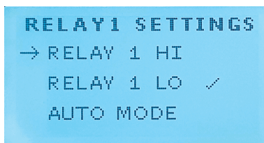
Fig. 59: Relay 1 Manual Operation
