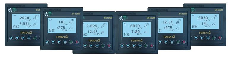
Measure two same or different parameters including pH, conductivity, and ORP with our **ATS-X2000 Series** dual-channel controllers. Their isolated design ensures superior noise control. Industry-acceptable control loop and relay logic makes them the ideal economical choice. These controllers offer set-point values and relays for High and Low digital control.
