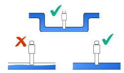
For accurate and stable readings, In a vertical line, sensor must be installed in a line where flow is upwards for improved contact and consistent flow.
