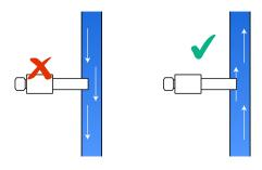
Sensor must be installed perpendicular to the line. Maximum angle of sensor to the line is 80°
